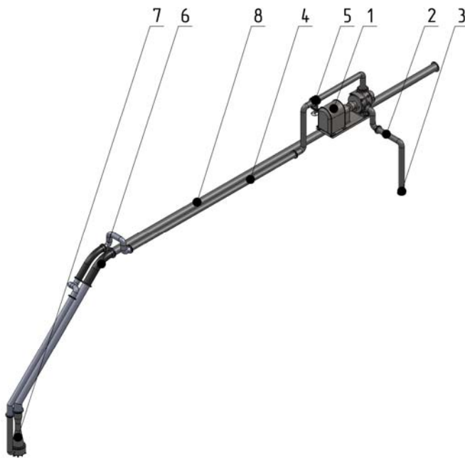
Fig. 1. Hydraulic system ejector pump dredger ZNS 300-120: 1 – water pump; 2 – intake pipe; 3 – back pressure valve; 4 – pump water conduit; 5 – doorbolt; 6 – flexible pipeline; 7 – draghead SGZ 300-120; 8 – dredging pipe
