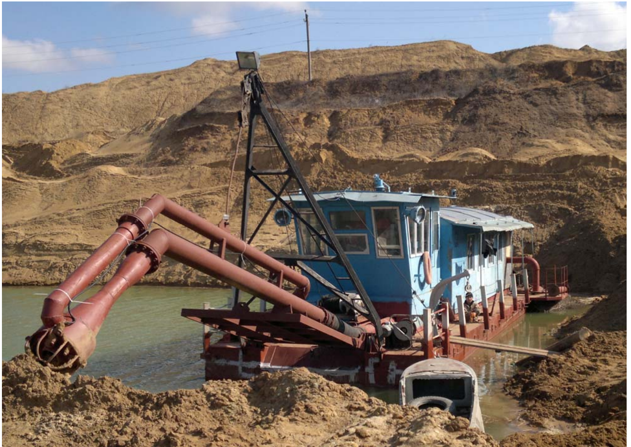
Fig. 2. Ejector pump dredger ZNS 300-120
